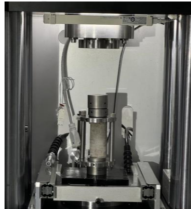
Uniaxial platen with strain gauges
