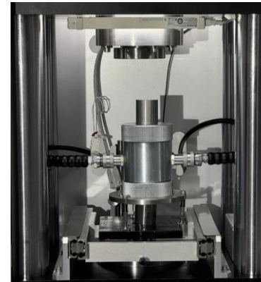
HOEK cell with strain gauges and Acoustic velocity fixture
