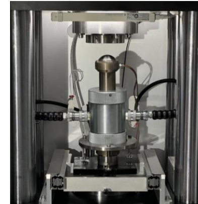
HOEK cell with strain gauges and Acoustic velocity fixture
