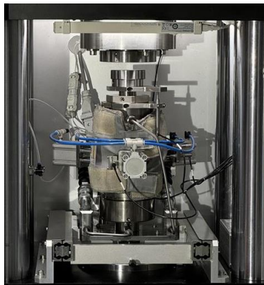
Triaxial load cell with strain deformation sensors
